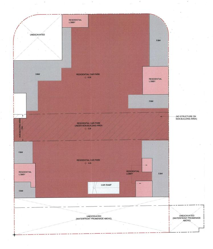
Master Layout Plan (Sheet 5 of 8) BASEMENT FLOOR PLAN (B/F)
